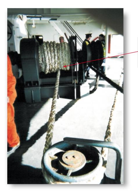
The starboard aft mooring winch was used to deploy the aft spring line. Note how the mooring rope leads from the underside of the drum.
