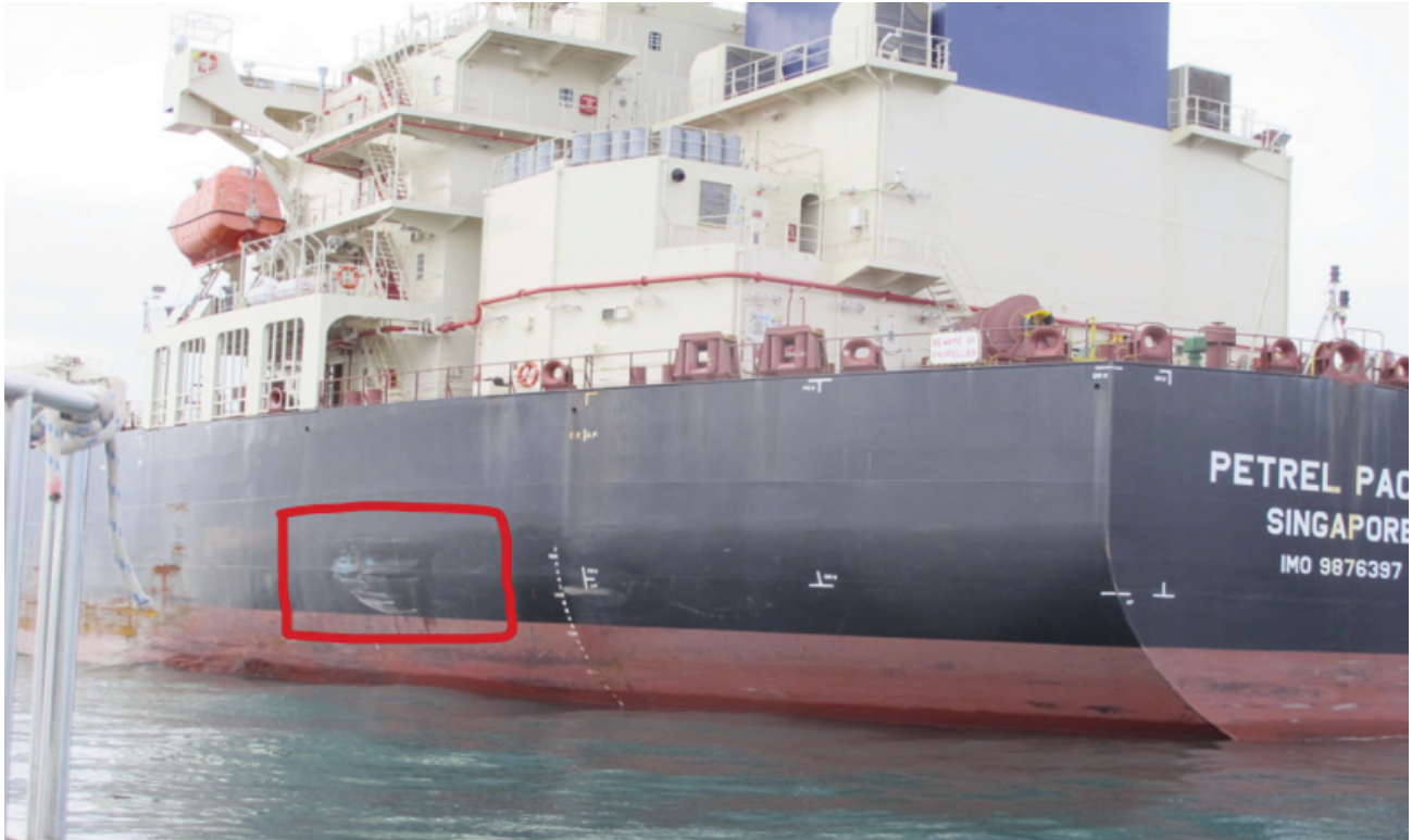
MV Petrel Pacific damage to port side shell plating.
