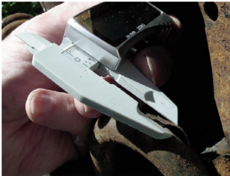
Photo 18 showing the width of the rupture.
