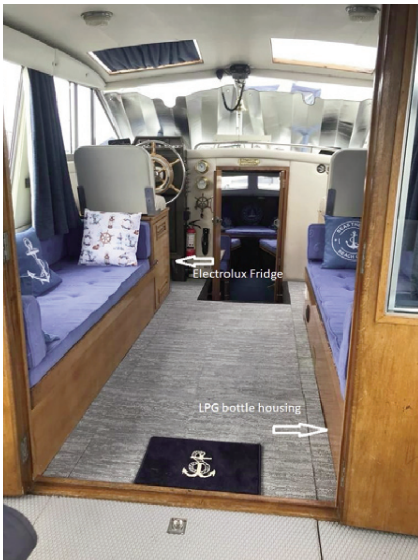
Photograph No.1: The interior of DollFinn looking forward showing the position of the fridge and the storage location of the LPG cylinders.
