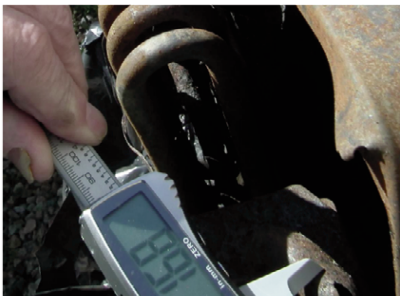
Photo 17 showing the length of the rupture as 16.8 mm.
