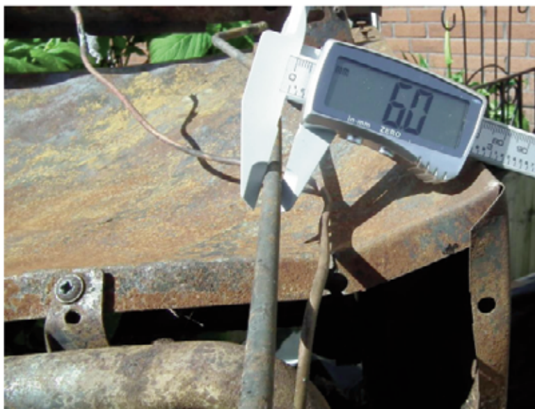
Photo 15 showing a view of the measured outside diameter of the gas supply pipe to the burner.
