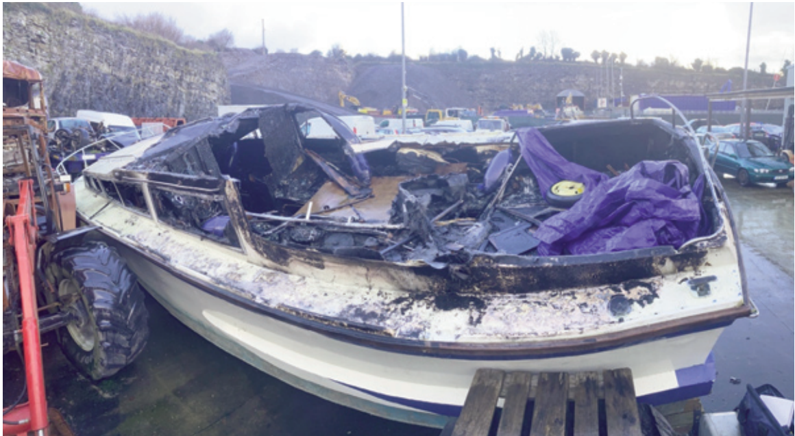
Photograph No.3: The remains of DollFinn clearly showing the extensive fire damage to the after section of the vessel.
