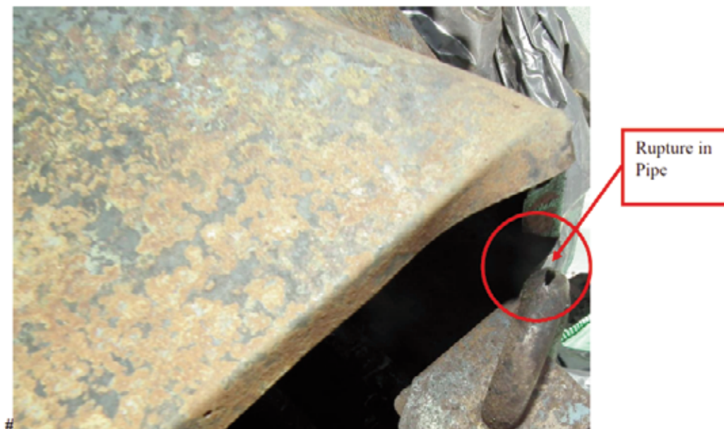
Photo 16 showing a view of a rupture in the ammonia circulation system.
