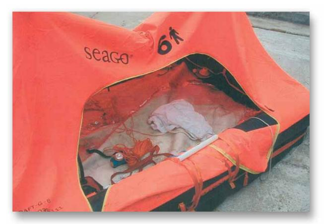
The interior of the liferaft with the floor insulation showing remnants of the aluminium outer cover that was removed by the survivors in an attempt to make a heliograph.
