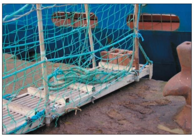
8.2.12 Gangway rigged after recovery wth safety net beneath.
