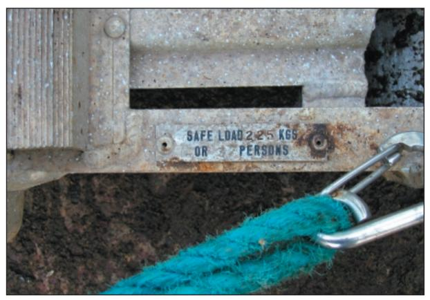
8.2.6 Side end of gangway. First set of stanchions not fitted, but roped off.
