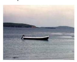
The vessel was defined as a 6 oar wooden Curragh. The build construction of the vessel is carvel built with  $^{3}/_{4}$  inch larch planking. The vessel had sawed oak frames. The hull was caulked with a tar film cover. The colour of the 'Curragh' was white at the gunwhales with a black hull.
