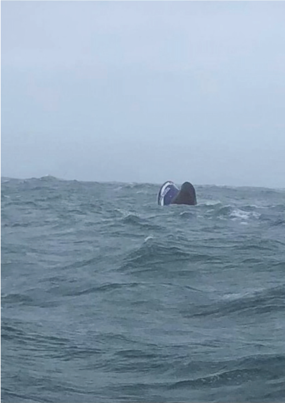
Appendix 7.32 A. Photograph of FV Ellie Adhamh showing the Bulbous Bow's Bulb in the Air as the Vessel Sank
