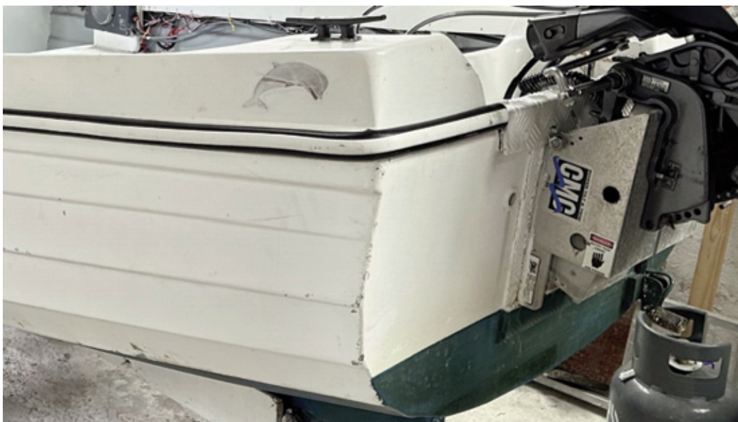
Figure 14: Aft of the Casualty's motor boat, with space available for the potential retrofitting of a reboarding ladder or an emergency overboard ladder.
