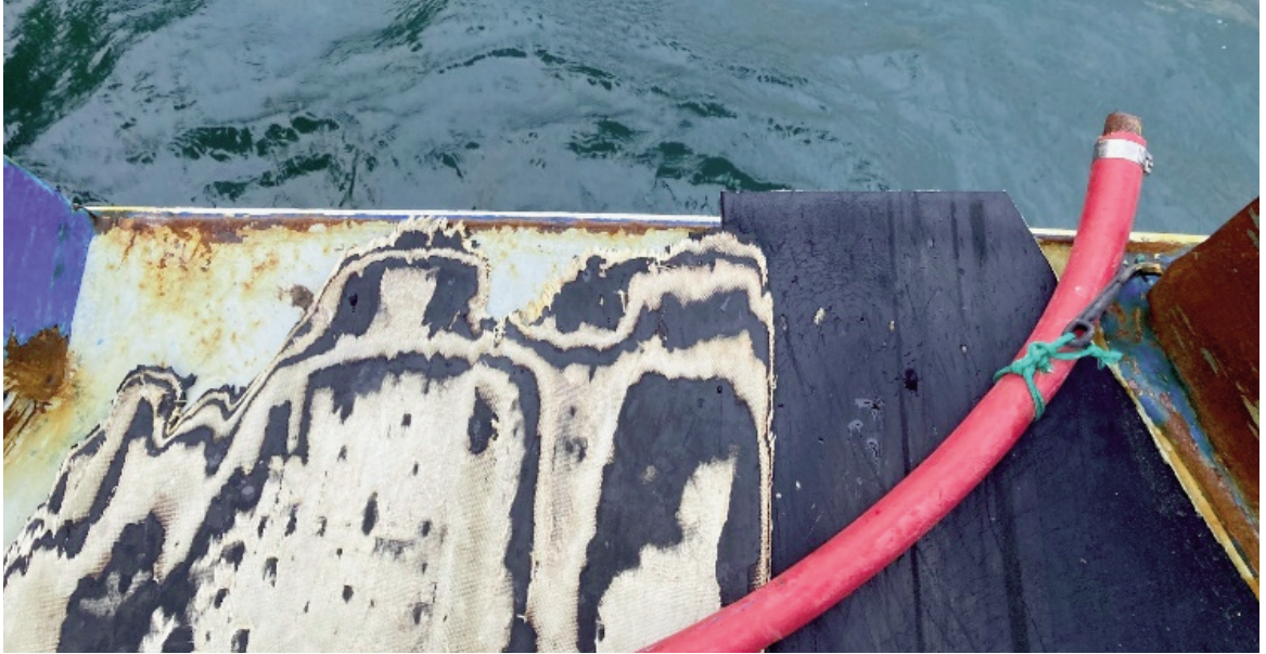
Photograph No.6: Deck edge at stern in way of stern door opening, the 90° edge chafed through the leader when the crew attempted to pull it back onboard.
