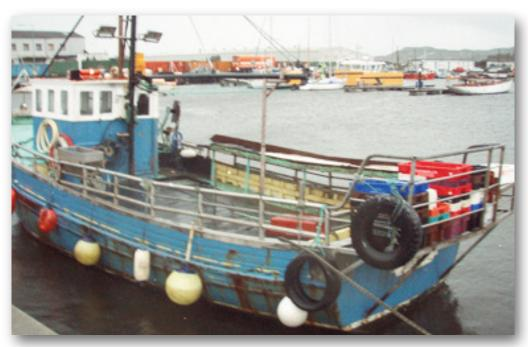
Photograph No. 2: The 'FV KERRI HEATHER' viewed from astern, note pot hauler and ramp on starboard side.
