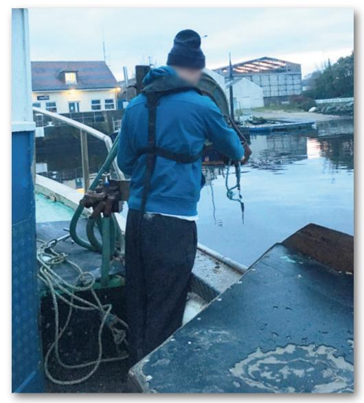
Photograph No. 3: Position of person at pot hauler when hauling pots. The anchor was reported to be on the ramp in foreground of the photograph. When falling forwards a person could hit their head on the hauler.
