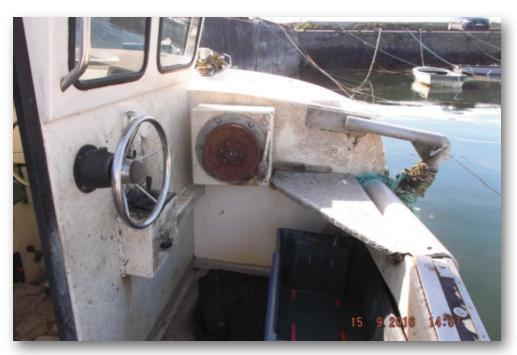
Photograph No. 5: Secondary controls beside pot hauling system.
