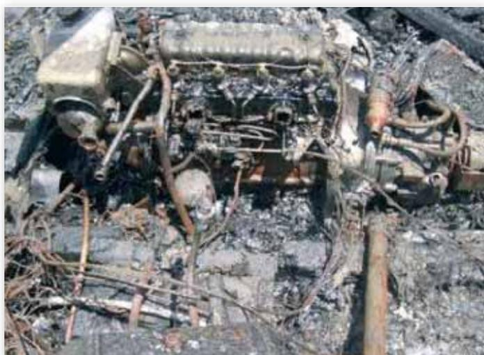
Photo 8 - Shows inlet manifold missing from engine
