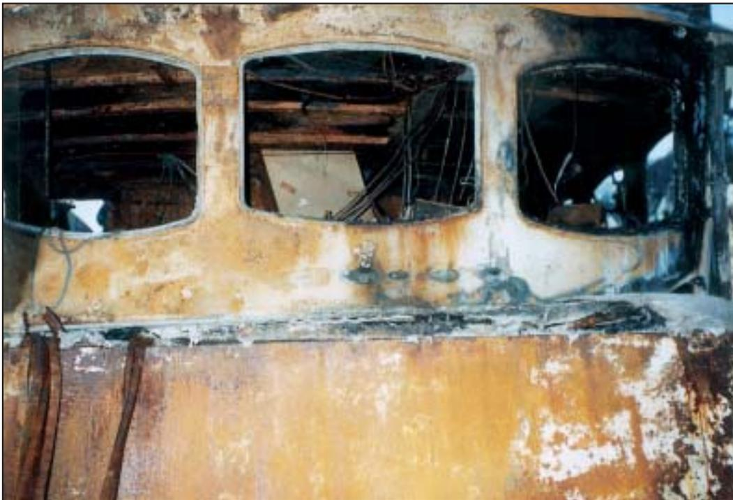
**Top:** Collapsed Shelter Deck and hydraulic oil hoses charred net bins.
