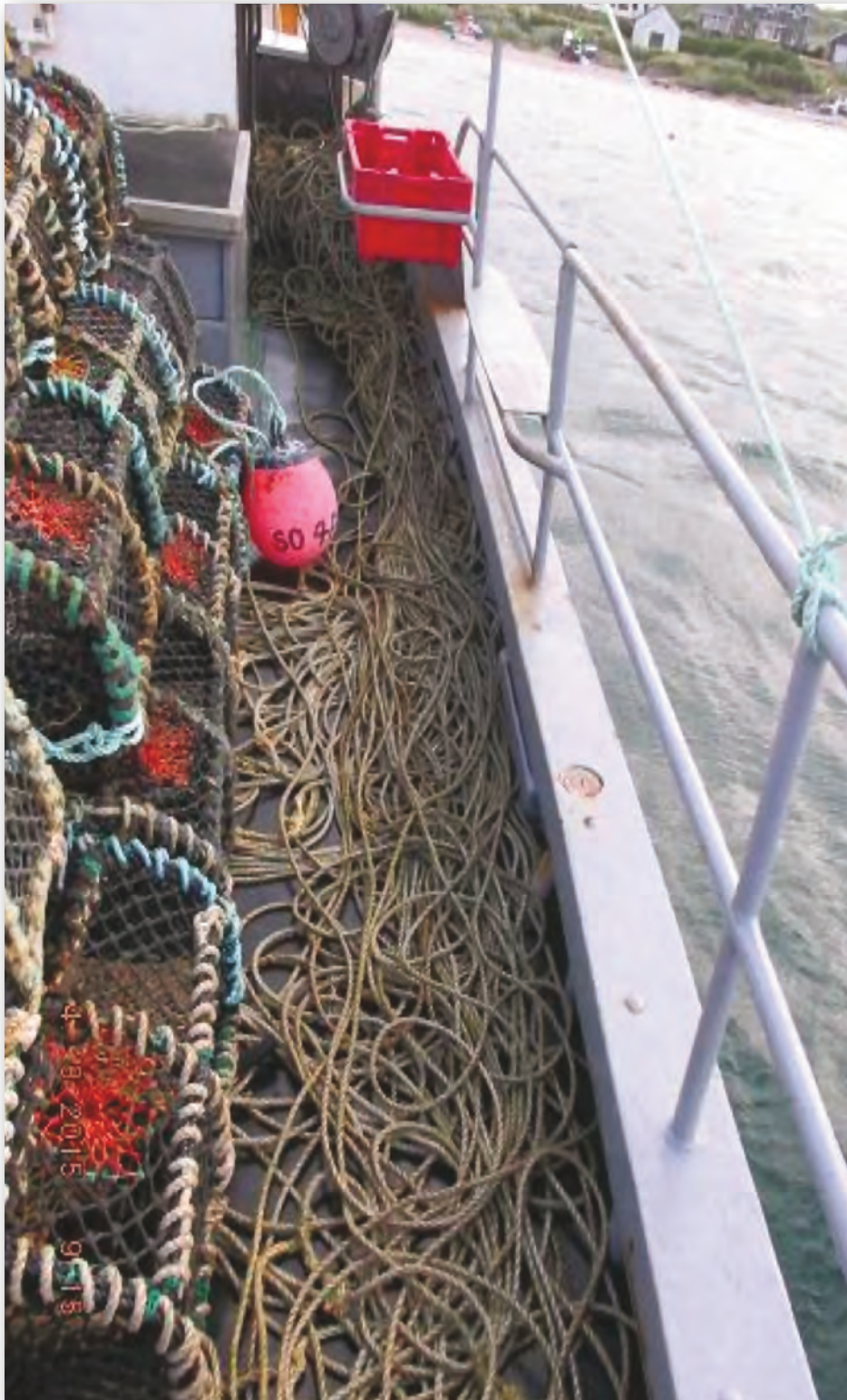
Photograph No. 5 - View along starboard side, fish box in cradle for catch and new top section of rail in place at opening for landing pots
