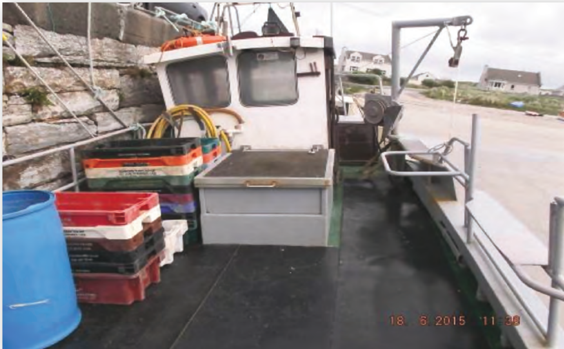
Photograph No. 1 - View from aft shows offset wheelhouse and pot hauler davit. Engine and fish hold hatch is immediately aft of the wheelhouse. Both aft windows are crazed from u/v light
