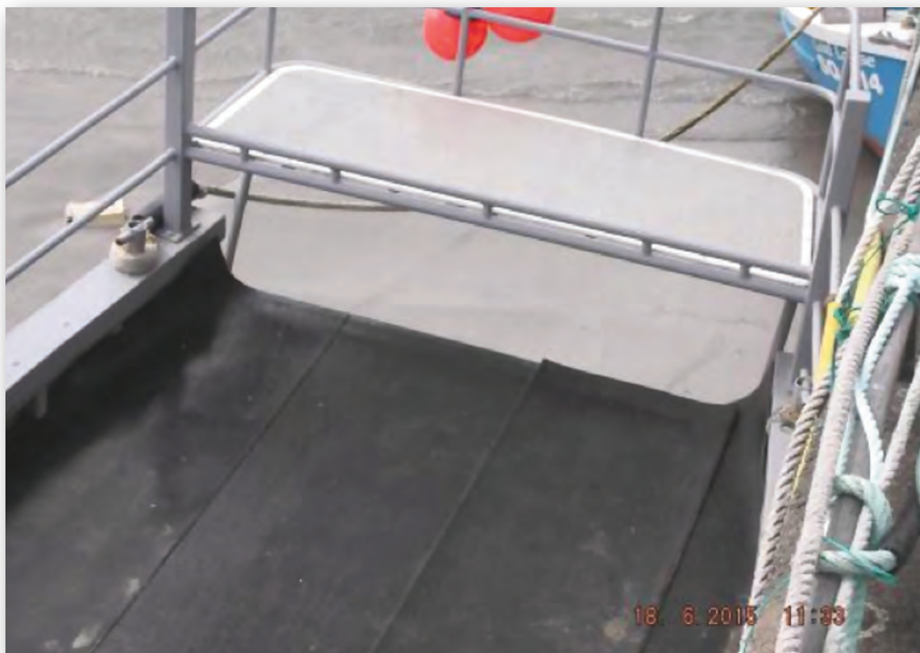
Photograph No. 2 - View of opening of transom and the conveyor belt rubber used on deck
