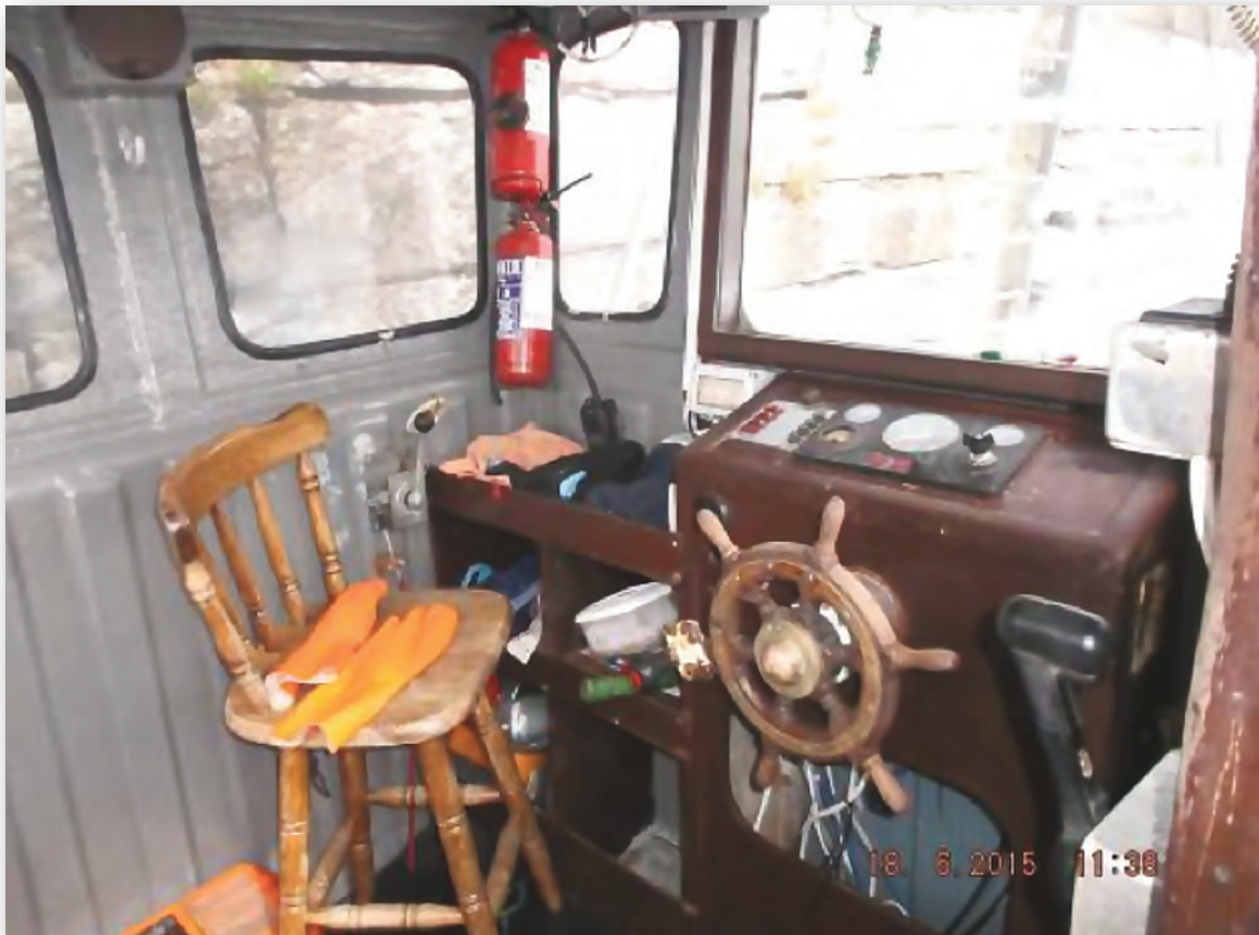
Photograph No. 8 - Inside wheelhouse. Engine throttle lever on right and hydraulic pump control on left beside chair
