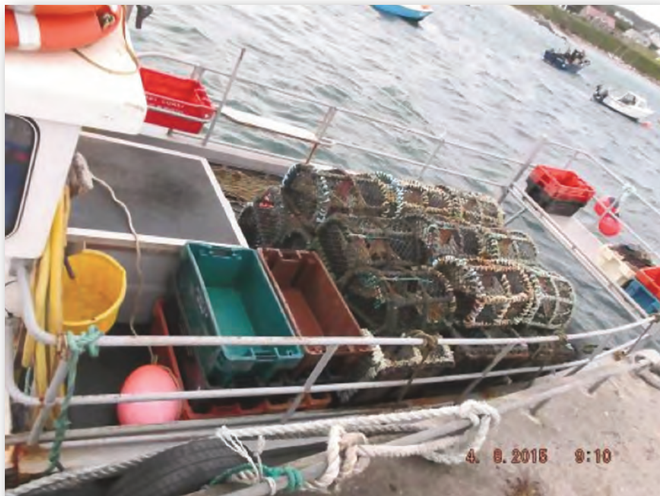
Photograph No. 4 - Vessel with pots set up for shooting string
