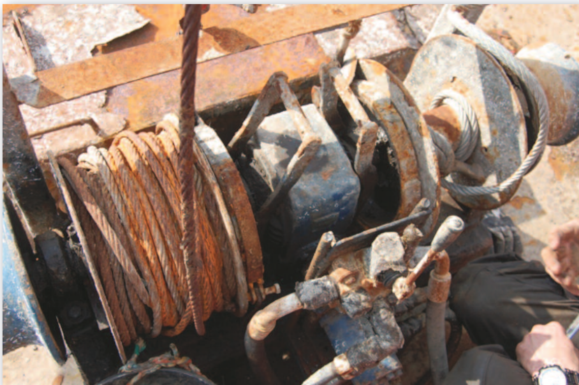
Photograph No. 8 - Showing the Dredging cage lifting winch with lifting line wound up
