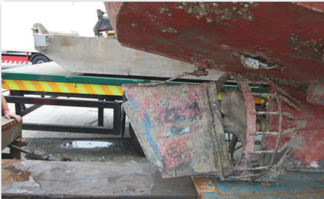
Photograph No. 3 - Showing damage to rudder and propeller
